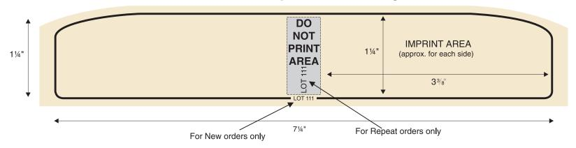
Due to new Federal Regulations we are required to put Lot #'s on all products and packaging. On all repeat orders we are punching out a section in the center of the plate and replacing it with a slug so that a new plate does not need to be purchased. For all new orders we are trying to put it in the border in the center at the bottom.
